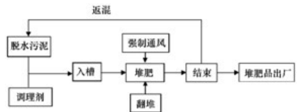
图1 强制通风槽式污泥生物干化流程示意 Fig. 1 Diagram of sludge bio-drying by continuous aerated and turning process
