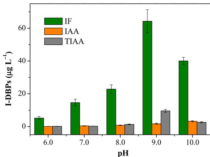
**Fig. 4.** Effect of pH on I-DBP formation during oxidation of IPM by Fe(VI). Experimental conditions:  $[\text{Fe(VI)}]_0 = 0.5 \text{ mM}$ ,  $[\text{NOM}]_0 = 0.5 \text{ mgC L}^{-1}$ ,  $[\text{IPM}]_0 = 50 \text{ }\mu\text{M}$ , reaction time = 72 h, 25 °C. Error bars represent the 95% confidence interval.
