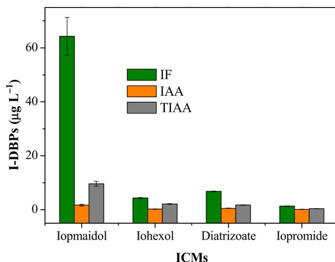
Fig. 7. Formation of I-DBPs during oxidation of different ICMs by Fe(VI). Experimental conditions:  $[\text{Fe(VI)}]_0 = 0.5 \text{ mM}$ ,  $[\text{IPM}]_0 = 50 \mu\text{M}$ ,  $[\text{NOM}]_0 = 0.5 \text{ mg L}^{-1}$ , reaction time = 72 h, pH 9.0, 25 °C. Error bars represent the 95% confidence interval.
