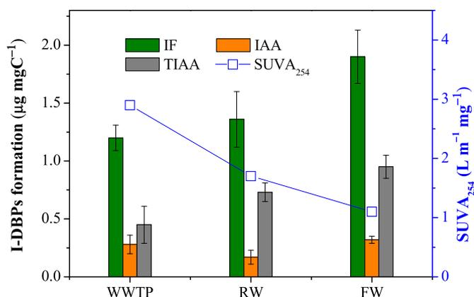
**Fig. 9.** Formation of I-DBPs during oxidation of IPM by Fe(VI) in real water samples. Experimental conditions:  $[\text{Fe(VI)}]_0 = 5.0 \text{ mg L}^{-1}$ ,  $[\text{IPM}]_0 = 500 \text{ } \mu\text{g L}^{-1}$ , reaction time = 72 h, pH 8.0, 25 °C. Error bars represent the 95% confidence interval. WWTP: wastewater treatment plant effluent; RW: river water; FW: filtered water in a drinking water treatment plant.
