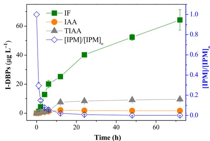
**Fig. 2.** Evolution of I-DBPs and normalized IPM concentration as a function of reaction time during oxidation of IPM by Fe(VI). Experimental conditions:  $[\text{Fe(VI)}]_0 = 0.5\text{ mM}$ ,  $[\text{NOM}]_0 = 0.5\text{ mgC L}^{-1}$ ,  $[\text{IPM}]_0 = 50\text{ }\mu\text{M}$ , pH 9.0, 25 °C. Error bars represent the 95% confidence interval.
