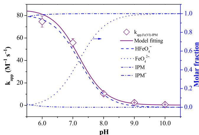
**Fig. 1.** Model fitting of the second-order reaction rate constant of IPM with Fe(VI) as a function of solution pH. Experimental conditions:  $[\text{Fe(VI)}]_0 = 0.1\text{--}0.5\text{ mM}$ ,  $[\text{IPM}]_0 = 10\text{ }\mu\text{M}$ , reaction time = 30 min, pH 6.0–10.0, 25 °C. Error bars represent the 95% confidence interval. IPM: iopamidol.
