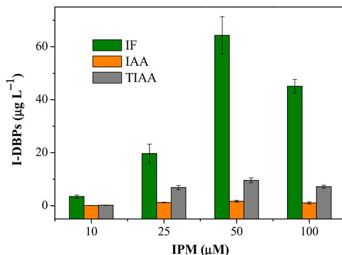
**Fig. 3.** Effect of initial IPM concentration on I-DBP formation during oxidation of IPM by Fe(VI). Experimental conditions:  $[\text{Fe(VI)}]_0 = 0.5\text{ mM}$ ,  $[\text{NOM}]_0 = 0.5\text{ mgC L}^{-1}$ , reaction time = 72 h, pH 9.0, 25 °C. Error bars represent the 95% confidence interval.
