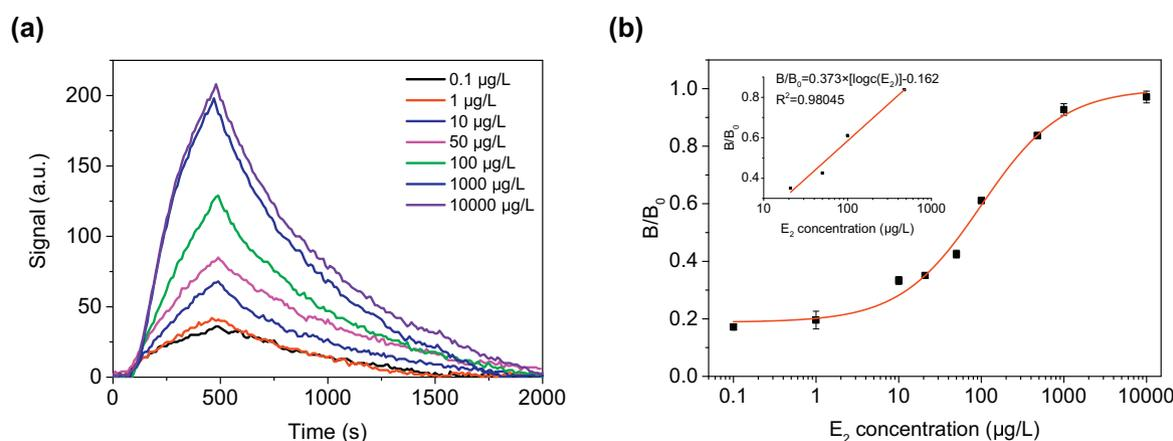
Fig. 5. (a) Original sensor grams of biosensor signals under different  $E_2$  concentrations and (b) variations of corresponding peak values and logarithmic fitted calibration plot. The inset depicts the linear range of  $E_2$  and corresponding calibration plot with the regression coefficient of  $R^2 = 0.98$ .
