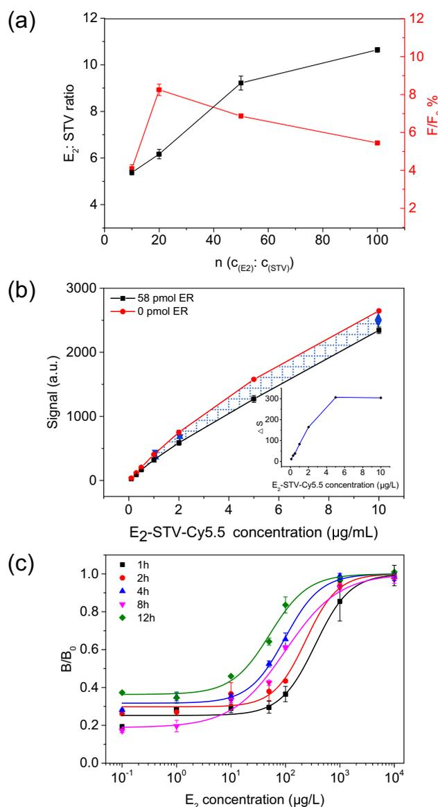
Fig. 4. Optimisations of detection performance: (a)  $E_2$ /STV ratio (signal recovery efficiency equals  $F/F_0$ , where  $F_0$  and  $F$  represent the initial fluorescent intensity and fluorescent intensity after adding  $E_2$ , respectively), (b) conjugate concentration and (c) affinity binding time.
