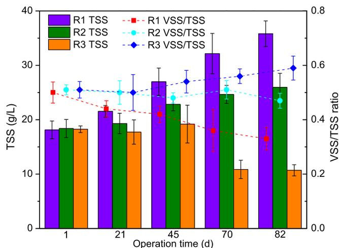
Fig. 3. Variation of TSS concentration and VSS/TSS ratio for DSR-EGSB reactors with different recirculation ratios of 3:1 (A), 6:1 (B) and 9:1 (C), respectively.
