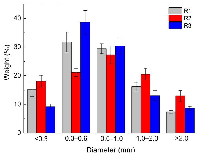
Fig. 4. Granule sludge size distributions by weight (sieving method) at the end of the operation.
