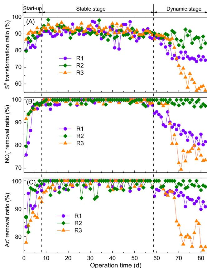
**Fig. 1.** Performance of the DSR-EGSB reactor at a recirculation ratio of 3:1 (R1), 6:1 (R2) and 9:1 (R3), respectively. (A)  $S^0$  transformation ratio; (B)  $NO_3^-$  removal ratio; (C)  $Ac^-$  removal ratio.
