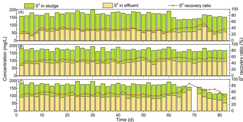
Fig. 2. Distribution of total produced  $S^0$  between sludge and effluent of DSR-EGSB reactors with different recirculation ratios of 3:1 (A), 6:1 (B) and 9:1 (C), respectively.
