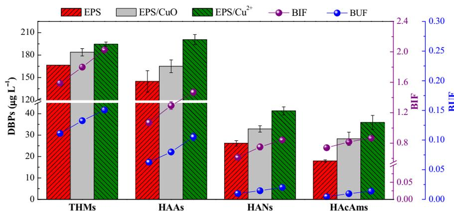
**Fig. 4.** Effect of  $Br^-$  on the catalytic formation of DBPs from EPS. Experimental conditions:  $[Cl_2]_0 = 9.8 \text{ mg L}^{-1}$ ,  $[EPS]_0 = 5.0 \text{ mg C L}^{-1}$ ,  $[CuO] = 2.0 \text{ g L}^{-1}$ ,  $[Cu^{2+}] = 2.0 \text{ mg L}^{-1}$ ,  $[Br^-]_0 = 1.0 \text{ mg L}^{-1}$ , pH = 7.6, reaction time = 72 h. Error bars represent the RPDs ( $n = 2$ ).
