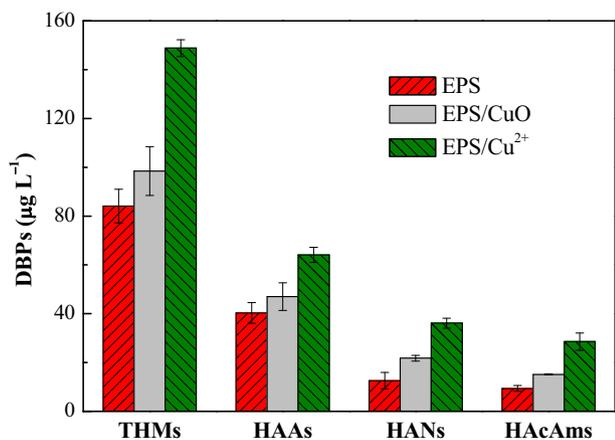
**Fig. 2.** Catalytic formation of DBPs from EPS. Experimental conditions:  $[\text{Cl}_2]_0 = 9.8 \text{ mg L}^{-1}$ ,  $[\text{EPS}]_0 = 5.0 \text{ mg C L}^{-1}$ ,  $[\text{CuO}] = 2.0 \text{ g L}^{-1}$ ,  $[\text{Cu}^{2+}] = 2.0 \text{ mg L}^{-1}$ ,  $\text{pH} = 7.6$ , reaction time = 72 h. Error bars represent the RPDs ( $n = 2$ ).
