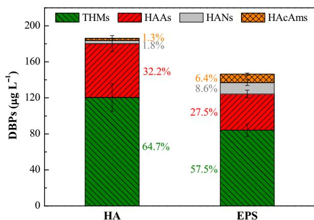
**Fig. 1.** Formation of carbonaceous and nitrogenous disinfection byproducts (C-DBPs and N-DBPs) from humic acid (HA) and extracellular polymeric substances (EPS) in the absence of copper corrosion products. Experimental conditions:  $[\text{Cl}_2]_0 = 9.8 \text{ mg L}^{-1}$ ,  $[\text{HA}]_0 = [\text{EPS}]_0 = 5.0 \text{ mg C L}^{-1}$ ,  $\text{pH} = 7.6$ , reaction time = 72 h. Error bars represent the relative percent differences (RPDs,  $n = 2$ ).
