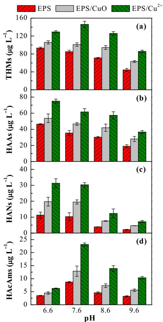
**Fig. 3.** Effect of pH on the catalytic formation of DBPs from EPS. Experimental conditions:  $[Cl_2]_0 = 9.8 \text{ mg L}^{-1}$ ,  $[EPS]_0 = 5.0 \text{ mg C L}^{-1}$ ,  $[CuO] = 2.0 \text{ g L}^{-1}$ ,  $[Cu^{2+}] = 2.0 \text{ mg L}^{-1}$ , reaction time = 72 h. Error bars represent the RPDs ( $n = 2$ ).
