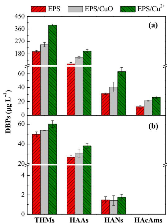
**Fig. 5.** Catalytic formation of DBPs from EPS proteins (a) and polysaccharides (b). Experimental conditions:  $[Cl_2]_0 = 9.8 \text{ mg L}^{-1}$ ,  $[Proteins]_0 = [Polysaccharides]_0 = 5.0 \text{ mg C L}^{-1}$ ,  $[CuO] = 2.0 \text{ g L}^{-1}$ ,  $[Cu^{2+}] = 2.0 \text{ mg L}^{-1}$ ,  $pH = 7.6$ , reaction time = 72 h. Error bars represent the RPDs ( $n = 2$ ).
