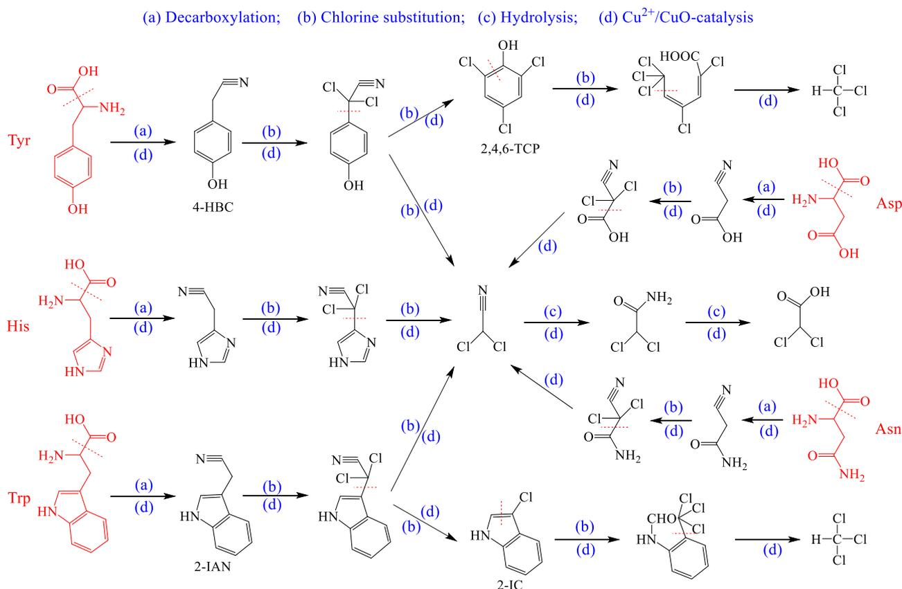
**Fig. 6.** Proposed mechanism of the catalytic formation of DBPs from amino acids. Experimental conditions:  $[\text{Cl}_2]_0 = 9.8 \text{ mg L}^{-1}$ ,  $[\text{Amino acids}]_0 = 3.0 \text{ mg C L}^{-1}$ ,  $[\text{CuO}] = 2.0 \text{ g L}^{-1}$ ,  $[\text{Cu}^{2+}] = 2.0 \text{ mg L}^{-1}$ , pH = 7.6.
