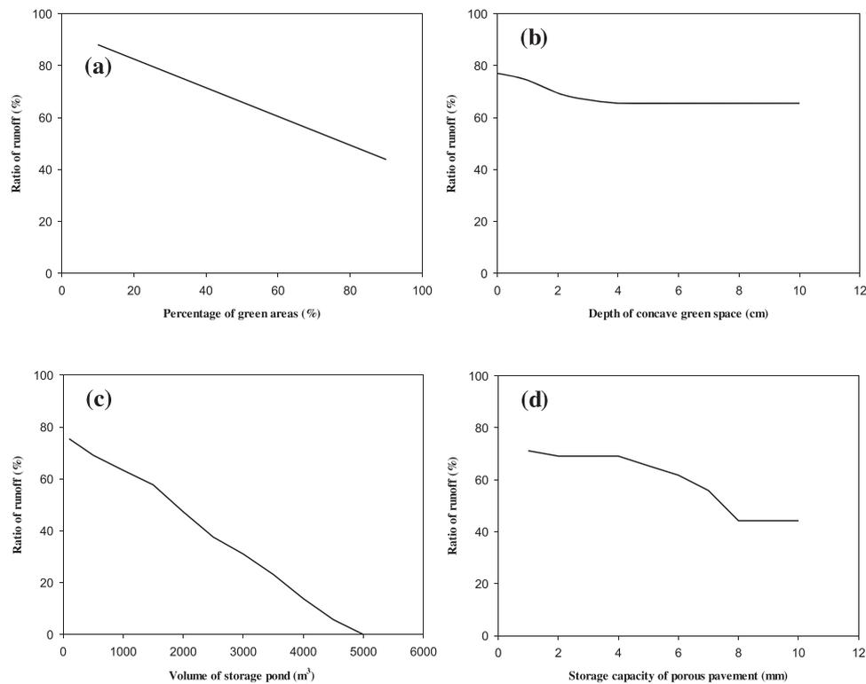
Fig. 4. Effects of setting sizes of single green infrastructure on runoff reduction.
