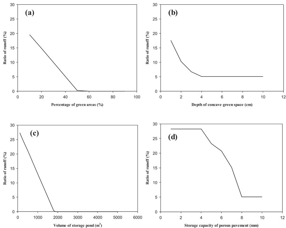
**Fig. 5.** Effects of setting sizes of green infrastructures on runoff reduction under the integrated scenario.
