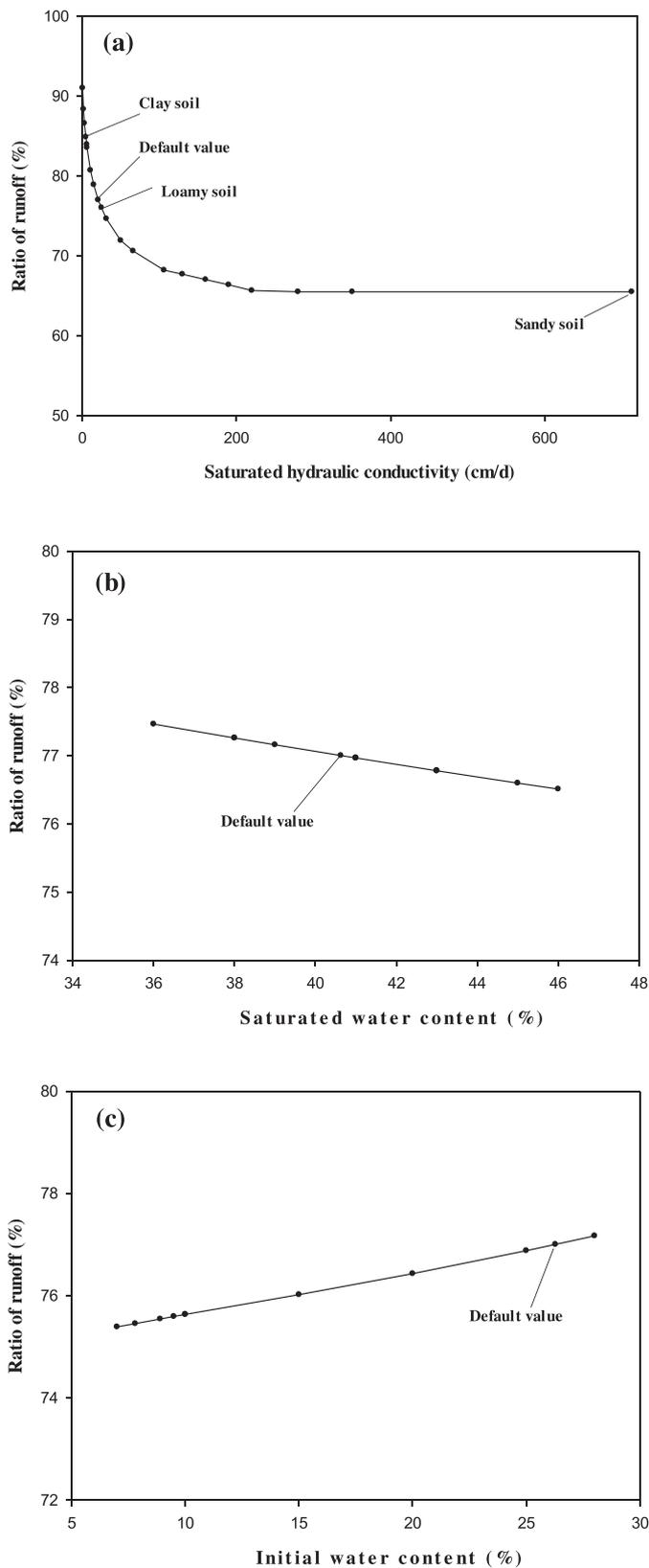
Fig. 3. Impacts of soil hydraulic parameters on the runoff to rainfall ratio.
