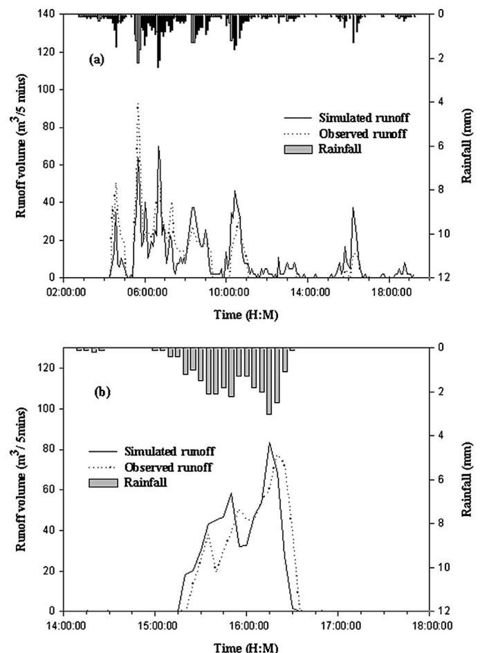
Fig. 1. Observed and predicted runoff hydrograph under: (a) rain event on July 15, 2013 (b) rain event on August 11pm, 2013.
