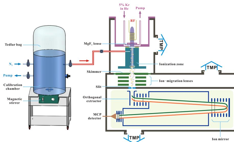
**Figure 1.** Schematic diagram of the calibration chamber and the AI ion source coupled with an orthogonal acceleration time-of-flight mass spectrometer.
