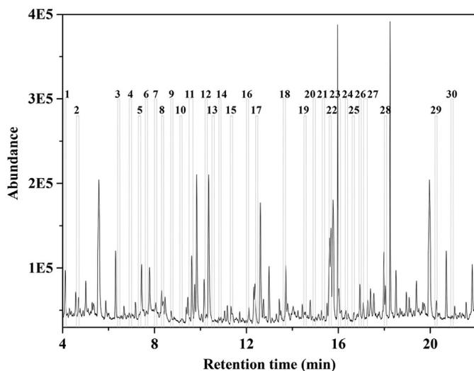
**Fig. 2.** Olfactogram overlaid on a GC/O chromatogram for source water of August in full-scan mode, pre-concentration method: LLE, pre-concentration factor: 1000, histogram: olfactory peaks, a total of thirty olfactory peaks were detected.
